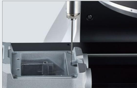
Even narrow locations are detected and measured automatically
