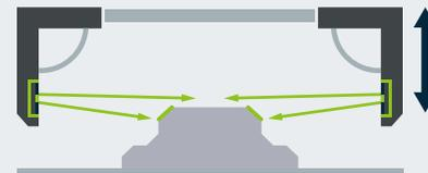
Narrow bands of light are projected horizontally. Place the illumination unit at the height of the edges to detect in order to create clear contrast at the desired location.
