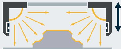
A wide area is illuminated. Placing the illumination unit at a high position illuminates the target evenly in its entirety. The lower the position, the greater the contrast in lighting due to height differences.
